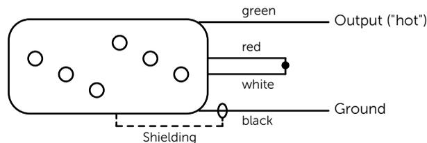
Because each coil picks up three of the six strings, a single-coil wiring - like with the Grand Vintage humbucker - is not possible. But you can connect the coils in parallel or stereo.
