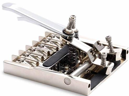
The **Duesenberg Multibender** enables you to play authentic sounding pedalsteel licks on nearly every normal electric guitar or lapsteel with a flat top. You can raise or lower individual strings from 1 to 3 half tones (depending on the string gauge used) by pressing with the palm of the right hand on one or more of the multibender's levers, which is normally done with a foot pedal or knee lever on a pedalsteel guitar.
