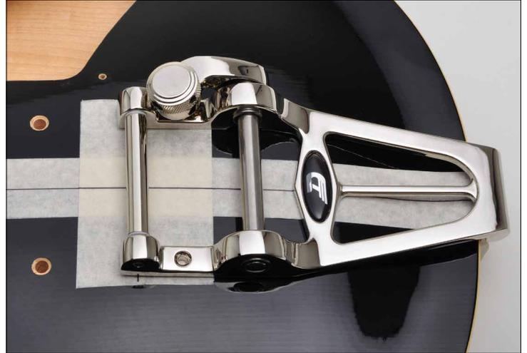
Next, position the two front mounting screws. The lateral position is adjusted by placing a thin thread into the nut and bridge notches of both E strings. The tremolo is then aligned side to side so that the thread has the same distance to both ends of the tension roller. Make sure that the tremolo is perpendicular to the center line. Then mark the positions of the screw holes on the top.
