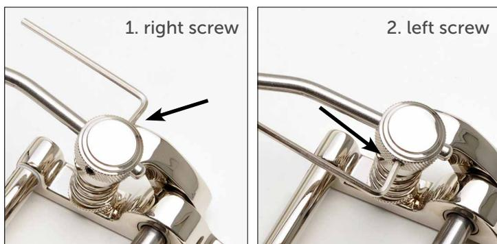
First tighten only the grub screw that has already been used to fix the arm in place. **Tighten this screw properly!** Only then the second screw is tightened. This prevents the lever from wobbling in the holder. However, the position of the lever can be corrected at any time later.
