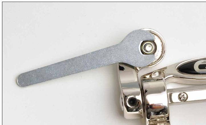
This nut will loosen a little at first. However, it can be readjusted at any time later. To do this, simply lift the arm so that you can remove the spring. The nut can then be adjusted with **the enclosed 8 mm wrench.**
