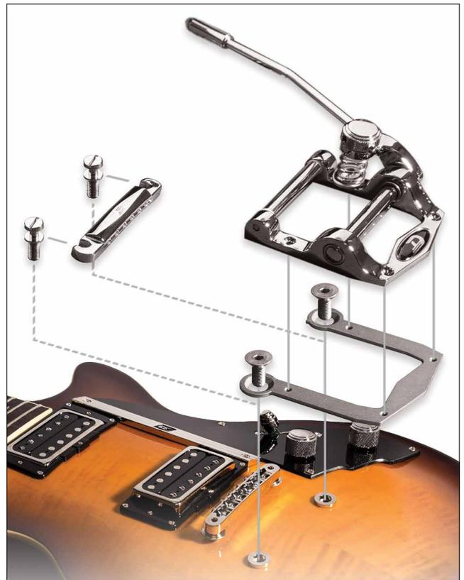
4. Put the Duesenberg Tremola onto the adapter and fix it with the M4 screws. The longest screw belongs under the tremolo's spring, which is on the right side on the right-hand version. Don't forget the spring support disk! The medium sized screw is installed on the other side of the tremolo and the two short ones on the back end, left and right of the D-Logo.
