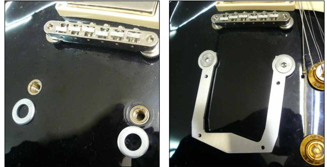
3. If necessary, put the washer onto the screw collars and install the Tremola Adapter using the fitting bolts. The countersink side of the large holes has to face upwards, so the mounting bolts flush with the adapter's surface. **Tighten the bolts sufficiently!**
