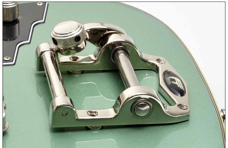
To reduce the angle, the tremolo is „jacked up“. To do this, place washers (e.g. the **Duesenberg Washer Set TDSWSN/TDSWSG**) under the frame of the tremolo at the two front mounting screws. The tremolo's rear edge rests on the top, which ensures a suitable contact angle for the strings.
